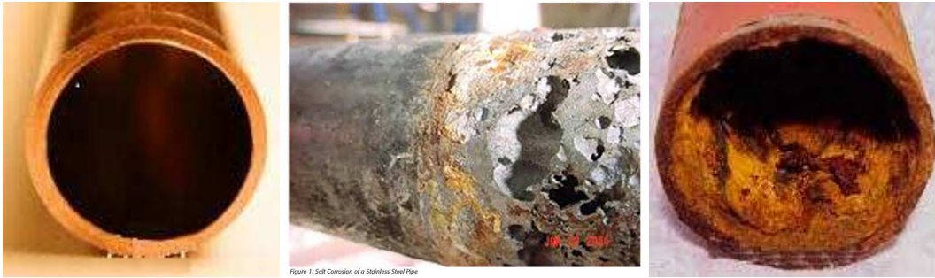
Figure 1: Salt Corrosion of a Stainless Steel Pipe
